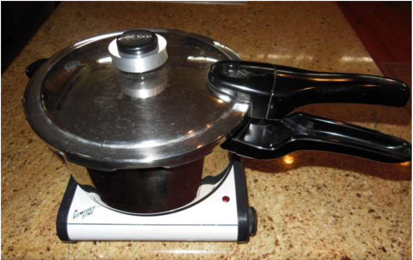
A four-quart, stainless steel, Presto Pressure Pot #01341 on an electric heater, with a CDS aluminum ring on the black regulator
