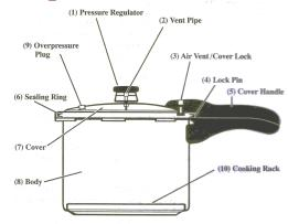
The ring weight increases the standard 16 pounds of cooking pressure to 24 pounds of pressure in the pot for absolute sterilization of your unbagged, unwrapped instruments.
